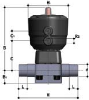
Pneumatically actuated diaphragm valve with male ends for solvent respectively socket welding, metric series , code 39, PVC-U, PP-H, PVDF, PVC-C
